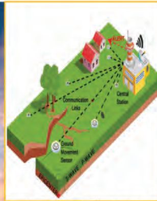
Implementation of an Earthquake Early Warning System based on the IoT and wave detection.
