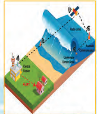
Implementation of a Tsunami Early Warning System based on the IoT and underwater sensors.
