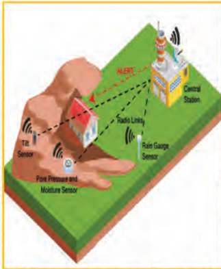
Implementation of a Landslides Early Warning System based on the IoT and underwater sensors.
